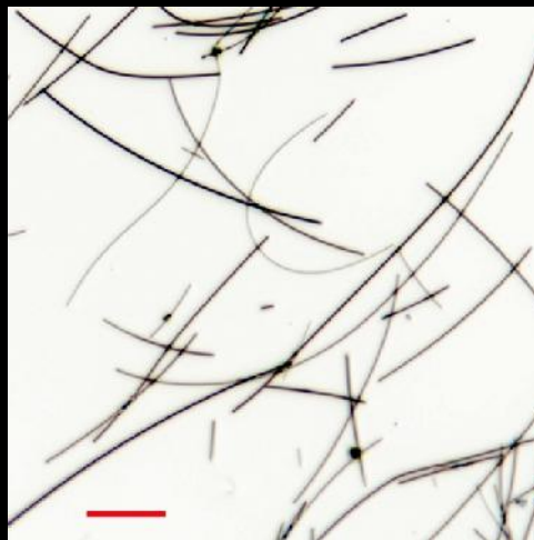
Silver Nanowires, Lot: ST475 Scale bar is 20 \mu m
